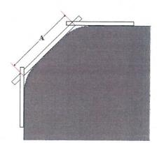
Using masking tape, simply extend the lines of your spa (or existing cover) as shown below. Where the tape intersects is where you want to measure out. In the diagram here, "A" is the measurement of the diagonal cut-corner. Alternately, a yardstick (or other small piece of wood) will also work.
