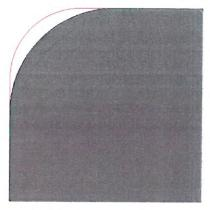
The diagram to the left shows the pitfalls of mis-measuring a rounded corner. The green line represents a measurement of too large a radius, while the red line represents a measurement too small. With too large a radius, the cover won't completely cover the spa. Too small a radius and the cover simply overhangs a bit. If in doubt, always go with a slightly smaller measurement. The cover may be slightly large and overhang the corner a bit, but it will cover the entire spa.
