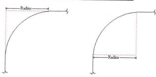
The diagram above shows a rounded corner with imaginary dotted red lines. The length of the red line represents the measurement of the radius corner. The lines start where the cover begins to curve, and end where they cross. Be sure to measure all corners and that they are ALL the same size! IMPORTANT: If in doubt, a smaller radius will slightly over hang the spa while a larger radius will not cover the spa completely.
