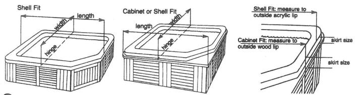
4 Cover Design and Taper: Bifold spa covers are tapered 4" to 2.5" for water run off. Bifold is how the majority of all spa covers are ordered. This design is available up to 96" x 96" in any shape. Quad-fold spa covers are a flat 4" thick for center panels with a 2.5" taper for outer panels and available up to 99" x 99" in any shape. Custom covers are available in multiple panels and larger sizes.
